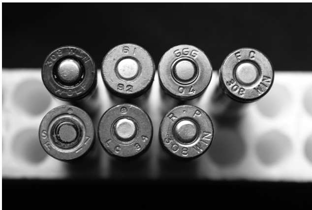
Figure 3.6 (See color insert.) An assortment of 7.6×51mm/.308 cartridge head stamps. Top row from left: Wolf Performance Ammunition; China State Factory 61; Giraites Ginkluotes Gamykla (2004); Federal Cartridge. Bottom row from left: Gevelot S.A.; Lake City Ordnance Plant; Remington Peters. (Image from author's collection.)
